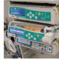
The pump is closed, and the display shows what type of syringe is in there. Settings can be adjusted.
